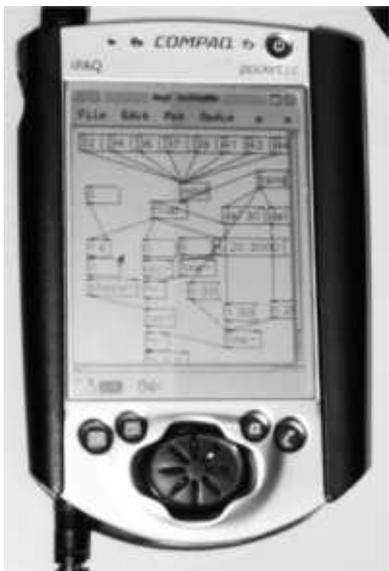
Figure 1: The iPaq running a PD FM synthesizer patch
